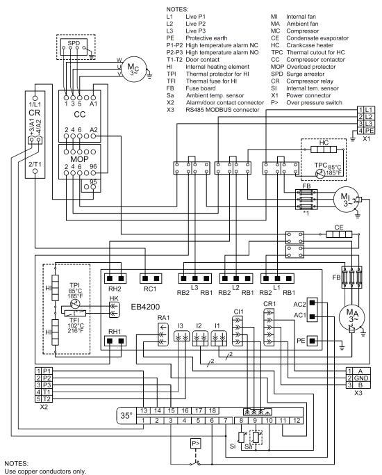
Use supply wires suitable for 75°C (167°F).
